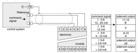
The option 4...20 mA uses the "0 mA" condition as breakdown-information. This means the presence of an evaluable failure information if the input signal line is interrupted. In this case the solenoid output will be switched off. The output will switched on when the input signal reaches a value of 3.8 mA, it switches
